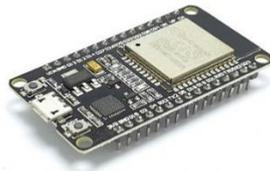
**Gambar 1** NodeMCU ESP32
