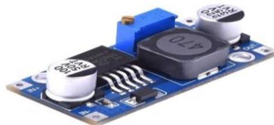
**Gambar 8** Step Down LM2596S DC to DC
